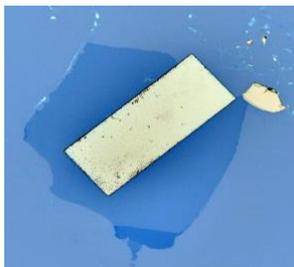
Figure 10: InGaAs emitter on top of the exfoliated graphene
