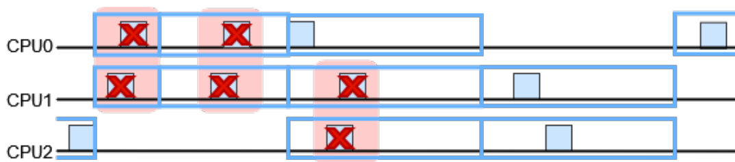
Figure 11: Timing diagramme of exponential backoff protocol. Red crosses mark colliding transmissions.
