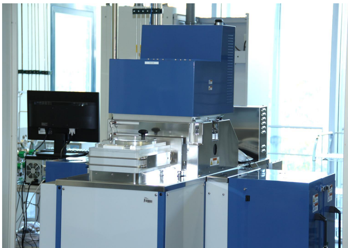
Figure 2. PECVD tool for graphene growth, located in the cleanroom of AMICA.
